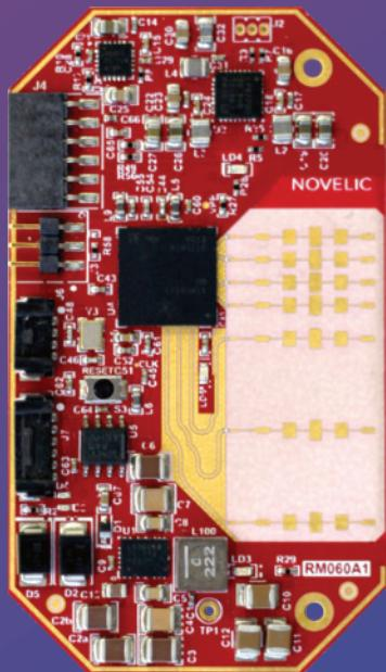
Unique! A **SIL 2, PLd, Category 3 Safety system** using a single-channel architecture for radar sensors
